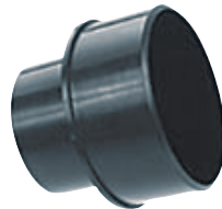
Stock number JW 1000, Reducer - Ø 100/57 mm Allows you to step down from larger main line to the machine to increase air velocity
